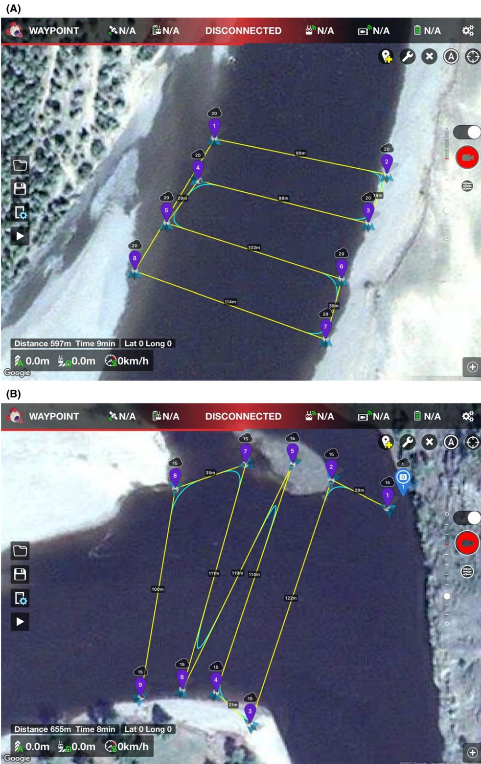
Figure 1. (A) Flight plan for the small unmanned aircraft system, showing the pre-programmed flight patterns and characteristics over Reach 1 (Uur River, Mongolia), which served as the low-probability Taimen environment; and (B) small unmanned aircraft system flight plan over Reach 2, which was an anticipated Taimen holding area.
